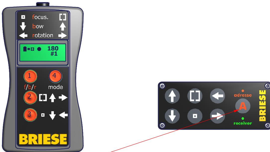
Confirm **A** on the E - Focus then choose address and radio frequency on the remote control. Enter "**LEARN**" with button 3. The red LED will blink 3 times on the E - Focus.
